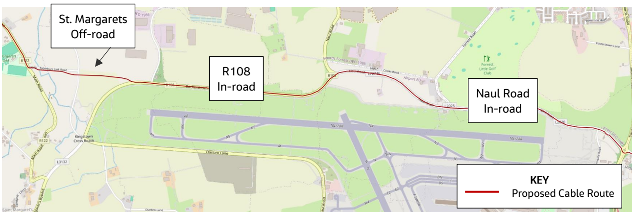
Image 6.7: Proposed Cable Route Along R108 Regional Road and Naul Road (North of Dublin Airport)
