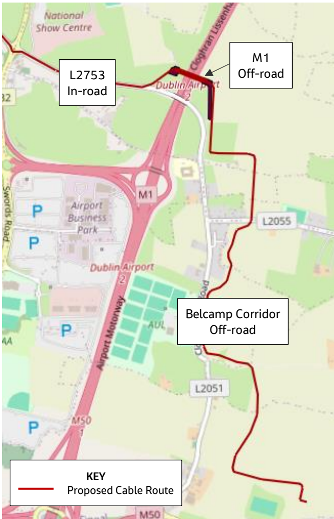
Image 6.8: Proposed Cable Route Along the L2753 Local Road, across the M1 Motorway to Belcamp Substation
